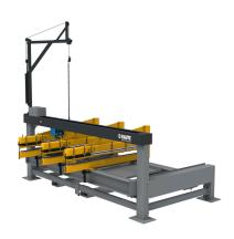
Proved to be the perfect solution for the panel quality control for Static load testing and impact load testing.
