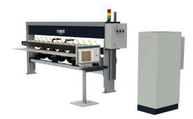
Analyzer with accurate moisture analysis of the veneers based on the contact brush moisture measuring to control the moisture of the veneer sheets going to the gluing process.
