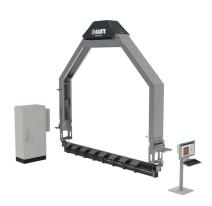
Analyzer with high-accuracy camera system and industrial light system to optimize defect detection for core veneer composing.
